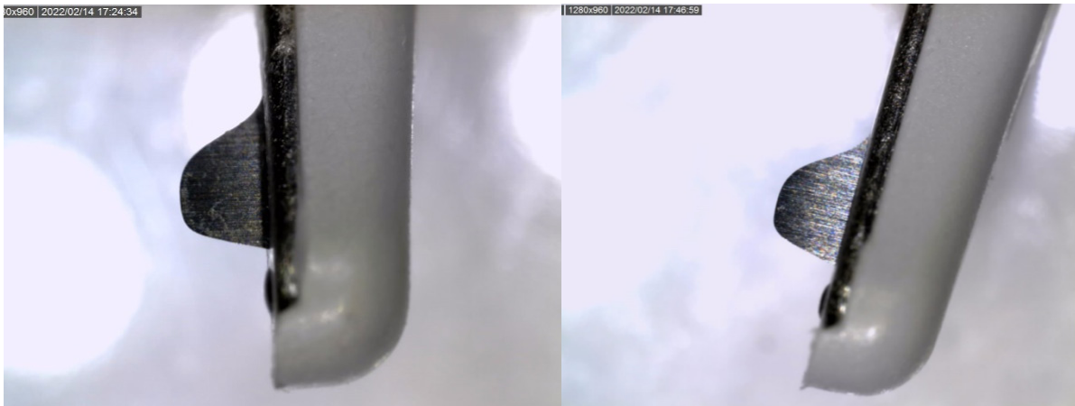
Figure 2. OM LF2019 blade vs. remanufactured LF2019 blade under magnification
